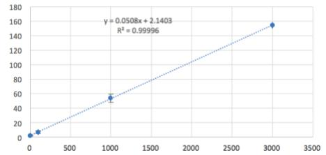
In our set-up, the true light intensity in  $\mu\text{mol photon m}^{-2} \text{s}^{-1}$  =  $0.0508 * \text{Blue Intensities} + 2.14$
