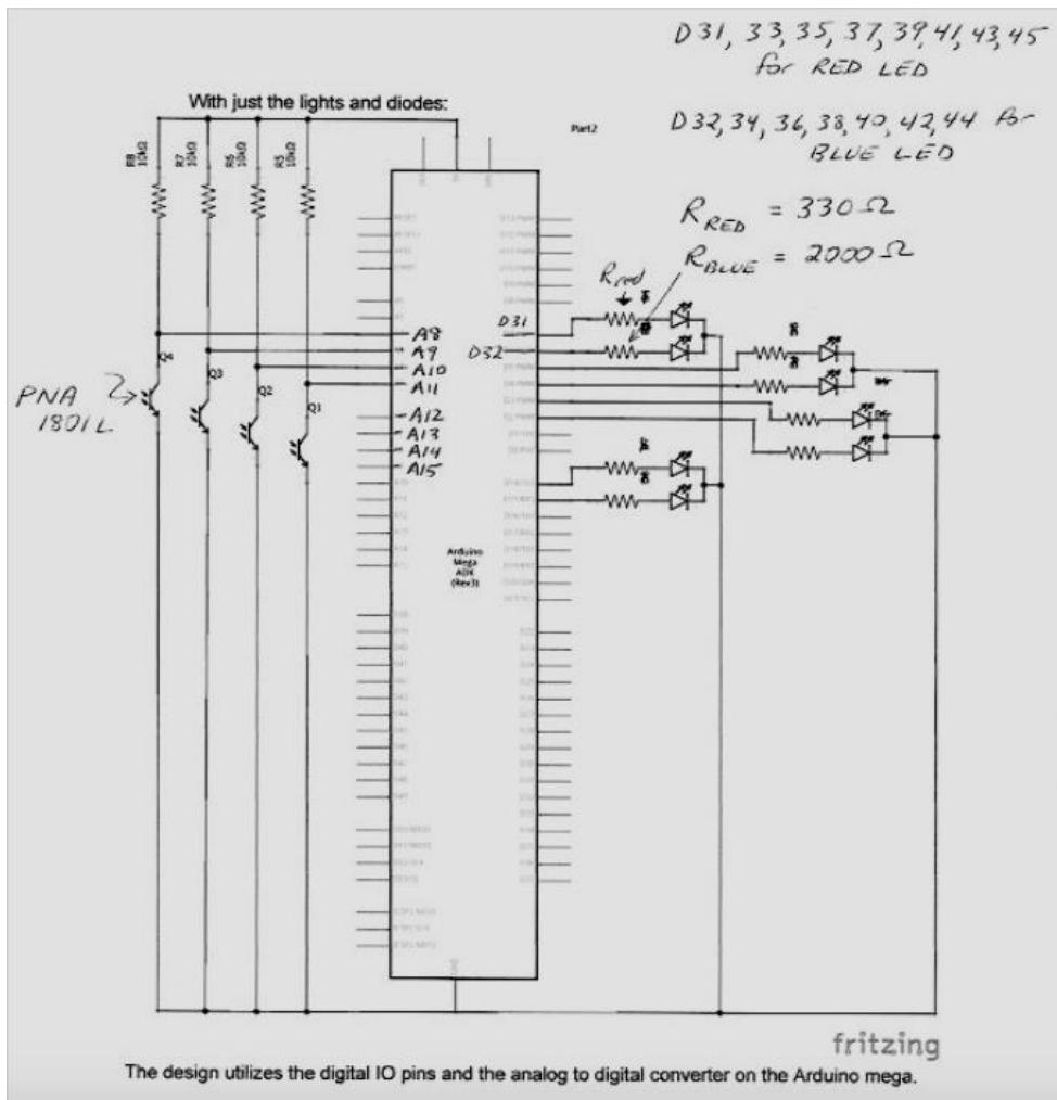
Eight phototransistors (PNA 180IL) are connected to A8-A15 and eight LEDs connected to pins D31-45 on the Arduino Mega 2560 as listed above in the wiring scheme.
